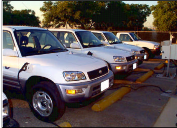
Figure 1. Some of Southern California Edison's Toyota RAV4s being charged with a Yazaki conductive connector.
